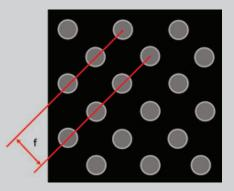
**Screen Frequency (lpi)** is the number of screen elements per inch, counted along a line where the elements are closest together. The diagrams in this document use f to designate this distance as it is also used to determine screen frequency. Screen frequency in lpi equals the inverse of distance f in microns multiplied by 25400.
