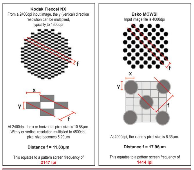
**Conclusion:** Although, no specific research has been completed to our knowledge, comparative experience tends to back up anecdotal evidence that finer patterns give superior results (smooth opaque ink solid ink transfer) from the range of relatively high-line screen anilox required to give high quality fine line and tone flexo printing.
